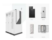
All-in-one energy storage system for commerce and industry; Comprises 60kW three-phase inverter and 200kWh advanced lithium-ferro phosphate (LFP) battery storage contained in a cabinet; Six MPP trackers with two strings per tracker; Maximum 200% PV oversizing input and up to 40A DC input current per MPPT; Global MPP scan for optimal energy harvest
