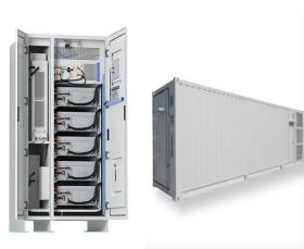
Build your Lithium Iron Phosphate (LiFePO4) battery bank with Victron's Smart Batteries. They are available in 12.8 and 25.6 Volts. Up to 20 batteries can be wired in series and parallel to configure your bank in 12V, 24V, or 48V nominal and to the desired capacity. Each cell in Victron's Smart Lithium Battery has a nominal voltage of 3.2V.
