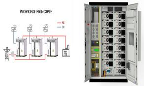
Improved Energy Efficiency. Hybrid inverters improve energy efficiency by storing extra solar electricity and reducing waste. Unlike traditional inverters, which only convert DC power to AC for immediate use, hybrid inverters also store surplus energy. This dual functionality prevents energy waste and ensures a continuous power supply.
