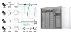
The PV inverter converts the direct current into alternating current, feeds the surplus energy into the grid and takes care of optimizing the energy: this is also possible without a battery inverter. A battery inverter by itself can only convert direct current from an electricity storage system into the required alternating current, thus it can
