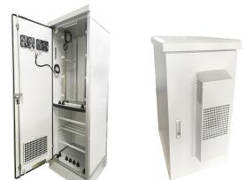
ESS-GRID series is BSLBATT's self-developed and manufactured pure battery system for commercial and industrial solar energy storage. The 100kWh battery system consists of 10 series-connected LiFePO4 51.2V 205Ah batteries a?|
