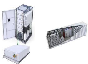
Pictured above, it has a total installed capacity of 30MW with 120 high-speed magnetic levitation flywheel units. Every 12 units create an energy storage and frequency regulation unit, the firm said, with the 12 combining to form an array connected to the grid at a 110 kV voltage level.
