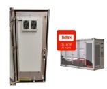
How much energy does a MTS tram use? In MTS trams,the Ni-MH battery features rated energy and power of 18 kWh and 85 kW,respectively,while the supercapacitors' rated power output is 288 kW. The total weight of the hybrid storage system is 1646 kg,resulting in specific energy and power of 11.45 Wh/kg and 226 W/kg,respectively.
