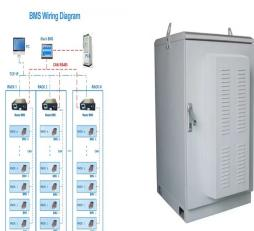
The BMS controls the flow of electrical energy into the battery pack to charge the cells efficiently. Efficiency investigation involves assessing charging energy losses. These a?|
