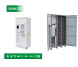
Jinko liquid cooling battery cabinet integrates battery modules with 1000V DC battery and capacity of 215kWh, and AC cabinet integrated with 100kW module PCS, transformer, etc. Also can be widely used in various application scenarios such as generation and transmission grid, distribution grid, new energy plants. APPLICATION
