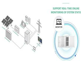
MEGATRON 50 to 200kW Battery Energy Storage Systems have been created to be an install ready and cost effective on-grid, hybrid, off-grid commercial/industrial battery energy storage system. Each BESS enclosure has a PV inverter making it easy for completing your renewable energy project (excludes MEG 200kW which is AC coupled).
