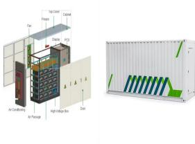
The Distributed Energy Storage solution powered by AI/ML uses the flexibility of backup power batteries to control electricity supply in thousands of base stations in the mobile network throughout the day. The DES system optimizes the timing of electricity purchases by scheduling charging and discharging periods for the batteries.
