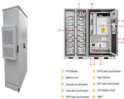
A battery energy storage system (BESS) contains several critical components. This guide will explain what each of those components does. The PCS has various modes which can be set for different charging and discharging strategies based on the specific application of the BESS. For the PCS or Hybrid Inverter to be effective within the BESS
