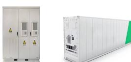
The Parker Outdoor Energy Storage PCS is equipped with a comprehensive list of protective devices for safe and reliable operation. DC Inputs: Contactor or circuit breaker disconnect, ground fault sensor, and surge suppression AC Output: Circuit breaker, phase current sensors (2), and surge suppression
