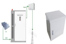
HOW OUR CONTAINERISED ENERGY STORAGE SYSTEMS WORK. Functioning like mini power stations, our battery storage containers (also known as BESS systems) load power from renewable energy sources into lithium-ion batteries, where it is kept until ready for future use.. A sophisticated battery management system oversees the a?
