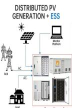
What is energy storage technology? The energy storage technologies provide support by stabilizing the power production and energy demand. This is achieved by storing excessive or unused energy and supplying to the grid or customers whenever it is required. Further, in future electric grid, energy storage systems can be treated as the main electricity sources.
