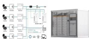
A hybrid energy storage system combined with thermal power plants applied in Shanxi province, China. Taking a thermal power plant as an example, a hybrid energy storage system is composed of 5 MW/5 MWh lithium battery and 2 MW/0.4 MWh flywheel energy storage based on two 350 MW circulating fluidized bed coal-fired units.
