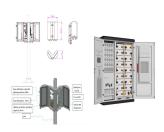
The project set out to address the requirement for short term energy storage with rapid charge/discharge cycling, typical of operation with renewable energy systems such as wind and wave. Flywheel kinetic energy storage is a suitable technology for use as a short term energy buffer, capable of high power transfer with continuous
