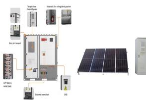
Peak regulation means that in order to alleviate the situation that the load rate of the generator set is lower than the prescribed range during the period of low load or the lack of positive reserve during the peak period, the power grid side energy storage accepts the dispatching instruction. the service provided by increasing or reducing
