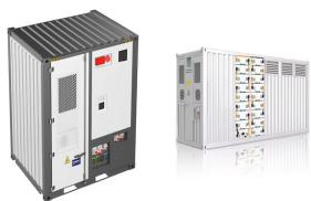
Energy storage converter. An energy storage converter, also known as a bidirectional energy storage inverter, English name PCS (Power Conversion System), is used in AC coupling energy storage systems such as grid-connected energy storage and microgrid energy storage to connect the battery pack and the grid (or load), it is a device that realizes two-way conversion of a?
