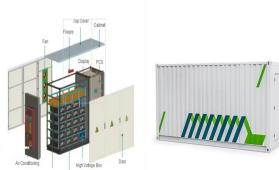
The SPICRI station is Chinas first power station with a hundred-kilowatt-level storage capacity. The rated output power and capacity of the energy storage demonstration power station are 250 kW and 1.5 MW.h, respectively. When operated commercially on large scales, the iron-chromium redox flow battery technology promises new innovations in
