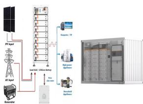
The RD-BESS1500BUN is a complete reference design bundle for high-voltage battery energy storage systems, targeting IEC 61508, SIL-2 and IEC 60730, Class-B. The HW includes a BMU, a CMU and a BJB dimensioned for up to 1500 V and 500 A, battery emulators and the harness. The SW includes drivers, BMS application and a GUI.
