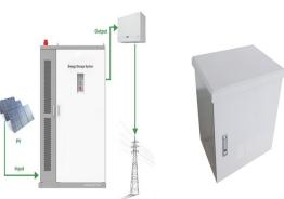
Battery storage is a technology that enables power system operators and utilities to store energy for later use. A battery energy storage system (BESS) is an electrochemical device that charges (or collects energy) from the grid or a power plant and then discharges that energy at a later time
