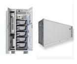
Batteries: Rechargeable battery units are the core of the Battery Energy Storage System. Battery units (often 20 ft. in length and 8 ft in width and height) include cooling systems to maintain optimal operating temperature. The cooling systems use fans and condensing units which can generate noise levels up to 92 dBA at 1 m from the equipment.
