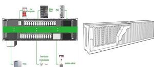
Nuvation Energy's High-Voltage BMS provides cell- and stack-level control for battery stacks up to 1500 V DC. One Stack Switchgear unit manages each stack and connects it to the DC bus of the energy storage system.
