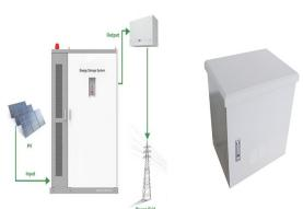
Solar photovoltaic (PV) power generation is the process of converting energy from the sun into electricity using solar panels. Solar panels, also called PV panels, are combined into arrays in a PV system. PV systems can also be installed in grid-connected or off-grid (stand-alone) configurations. The basic components of these two configurations
