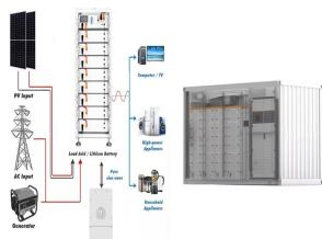
2 The most important component of a battery energy storage system is the battery itself, which stores electricity as potential chemical energy. Although there are several battery technologies in use and development today (such as lead-acid and flow batteries), the majority of large-scale electricity storage systems
