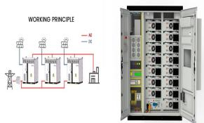
Socomec's outdoor energy storage solutions ensure the proper energy mix of buildings and the power grid's stabilization, making them ideal for commercial and industrial facilities. Discover our solutions to reduce energy costs, improve the resilience of the electricity grid or facilitate access to electricity: storage converters (connected and standalone), multi-technology batteries
