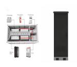
Common Method of Grounding for Photovoltaic Lightning Protection. For the solar panel grounding, general use 40 \* 4mm flat steel or ??10 or ??12 round steel, and finally buried depth of 1.5m underground, the grounding resistance of the ???
