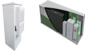
Hotstart's liquid thermal management solutions for lithium-ion batteries used in energy storage systems optimize battery temperature and maximize battery performance through circulating liquid cooling. Hotstart's engineered liquid thermal management solutions integrate with the battery management system (BMS) of a BESS to provide active
