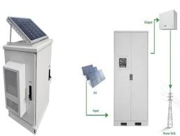
According to the requirements of grid dispatching or local control, the PCS charges the battery pack with AC power from the grid and can also discharge the energy storage battery. During peak grid load periods, the PCS inverts the DC power of the energy storage battery into AC power and feeds it back to the public grid; it also feeds or absorbs
