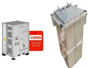
S90 energy storage cabinet is an all-in-one outdoor cabinet system containing bi-directional energy storage inverter module, DCDC PV optimizer module, STS intelligent switching module, battery system, transformer, fire protection system, air conditioning system, auxiliary source power supply and other energy storage batteries.
