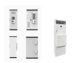
The SMA Sunny Boy SB7.7 is a 7,700 watt AC output grid-tied PV solar inverter that features 3 independent MPPT channels, a 2,000 watt off-grid secure power supply, lifetime monitoring, and an integrated DC disconnect safety switch. The SMA ???
