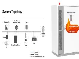
Comprehensive Container-Based Energy Storage System The container-based power station energy storage system integrates battery modules, battery management, monitoring, and auxiliary systems within a single containerized solution. This all-in-one design enables a wide range of applications, includ
