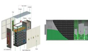
Utilizing standardized shipping containers as the housing for energy storage units facilitates transportation, installation, and deployment. The system allows flexible configuration of multiple energy storage units to meet various scale and power requirements in different application scenarios. Paragraph 3: Application Prospects;
