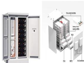
Outdoor energy storage cabinet, with standard configuration of 30 kW/90 kWh, is composed of battery cabinet and electrical cabinet. It can apply to demand regulation and peak shifting and C& I energy storage, etc. Split design concept a?|
