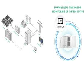
Off-grid inverters, known as stand-alone inverters, need a battery bank to function. When selecting off-grid solar inverters, it is essential that the output power of the inverter is large enough to support the loads of the system. Many off-grid solar inverters include a charger in order to replenish the battery.
