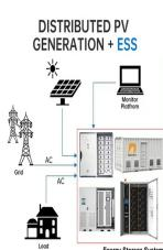
Distributed ESSs (Energy Storage Systems) in combination with advanced power electronics provides a solution for such problems. For these reasons the importance of UPS (Uninterrupted Power Supplies) and ESSs will increase in the near future. Commercially available ESSs beyond lead acid batteries offer alternatives for UPS and can introduce
