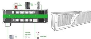
6 . I was the engineer in charge of installing and configuring this system in Yemen so I would like to share my experience. The old solar system was upgraded by adding a Fernius Eco inverter in the output of victron inverters/chargers. System Components: Victron side: Inverter/Charger 3 Quattro 10KVA, 48V, 240V (30 KVA-3 phase) PV panels 60 TrinaSolar a?|
