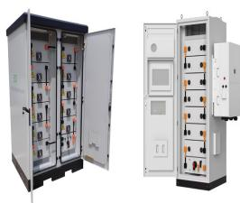
The VoltStorage VDIUM C50 is a 50 kWh redox flow battery storage system designed for self-consumption optimization in industrial, commercial, and agricultural applications. It can charge in 5-10 hours and discharge power for up to 10 hours, with a maximum AC charge power of 10 kW and discharge power of 9 kW. The long-lasting system has a lifespan of over 10,000 charge ???
