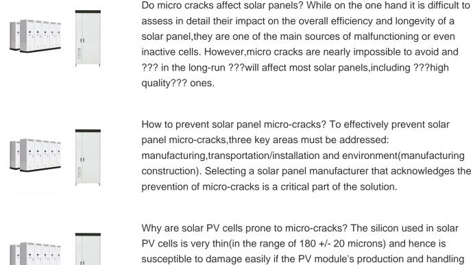
PV cells is very thin(in the range of 180 +/- 20 microns) and hence is susceptible to damage easily if the PV module's production and handling are not up to the required standards. Even slight imperfections in the PV cell can lead to large micro-cracks once it is incorporated into the PV module.
