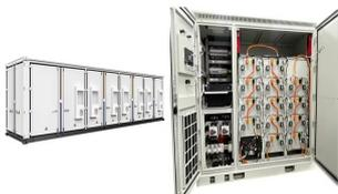
A modular LFP outdoor battery storage system . With EnerOne, CATL have designed an outdoor liquid-cooled battery energy storage system (BESS) based on lithium iron phosphate (LFP) cells. Nominated for an ess Award 2022, the EnerOne from CATL has a nominal storage capacity of 372.7 kilowatt hours with a foot print of just 1.69 square meters
